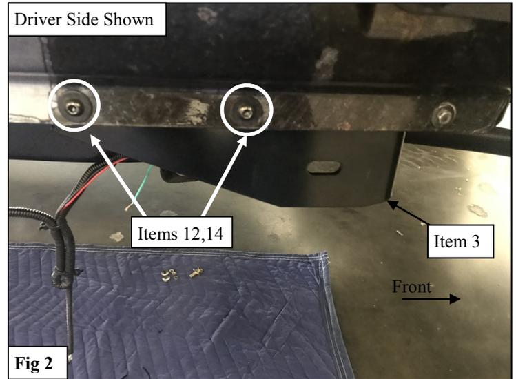
2. Loosely attach the Rear Mounting Bracket (5,6) to the vehicle's pinch weld and frame using the supplied M8 Hardware.
